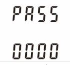
Setting up is password-protected so you must enter the correct password (default '1000') before processing. If an incorrect password is entered, the display will show: Err
