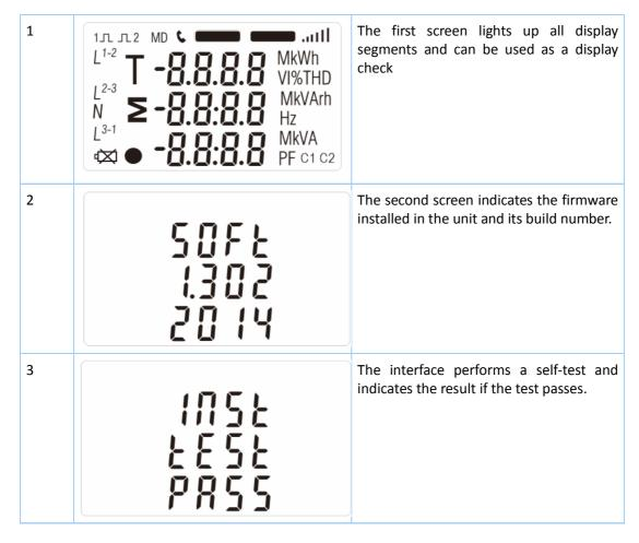
After a short delay, the screen will display active energy measurements.
