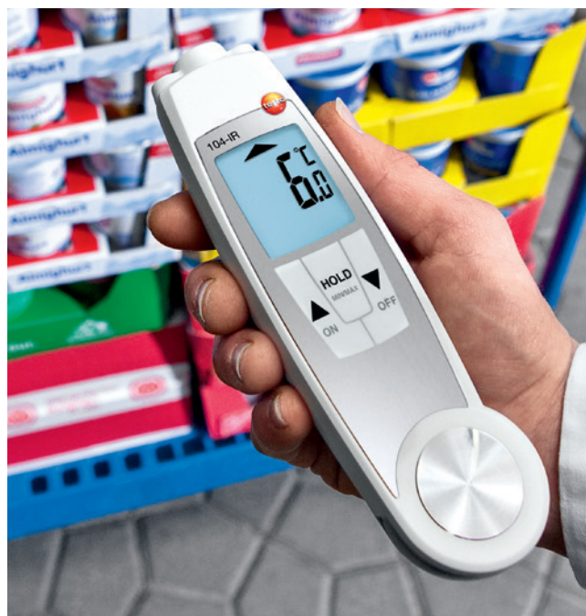
Checking temperature in Incoming Goods with testo 104-IR
