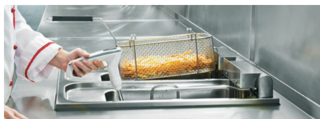
Measuring cooking oil quality with the testo 270
