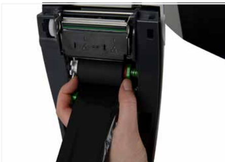
Insert the entire core of the ink ribbon at the bottom.
