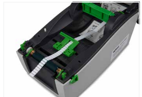
Loosely fit guide rails to the material.
