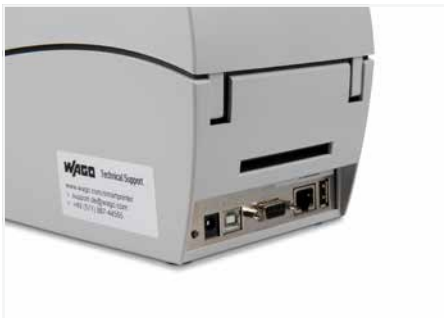
Secure Bluetooth® (258-5102) or WiFi Dongle (258-5103) in the USB-A interface.
