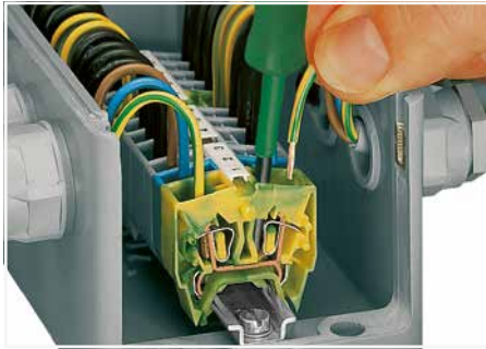
CAGE CLAMP® termination: Inserting a conductor. With ferruled conductors, it is necessary to use a terminal block one size smaller than the conductor's nominal cross section.
