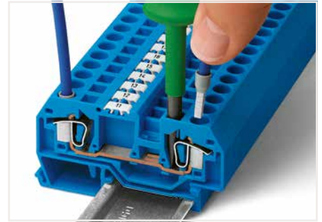
CAGE CLAMP® connection Inserting a conductor. With ferruled conductors, it is necessary to use a terminal block one size larger than the conductor's nominal cross-section.
