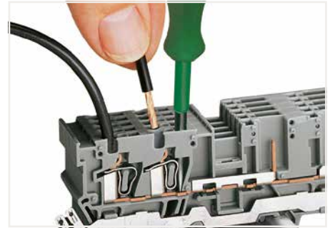
Carrier terminal block: Insert/remove conductor via operating tool (3.5 x 0.5 mm blade).
