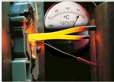
Glow-Wire Test per IEC/EN 60998-1, IEC/EN 60695-2-11
