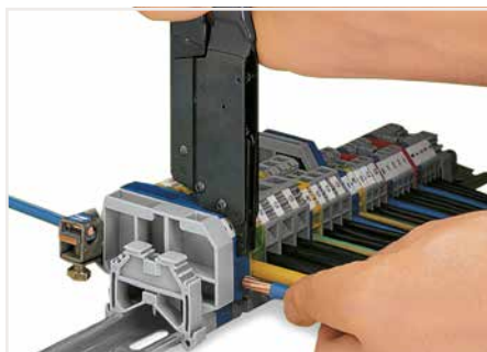
When operating the handles beyond the locked position, the ratchet allows the tool to open and be removed from the terminal block.
