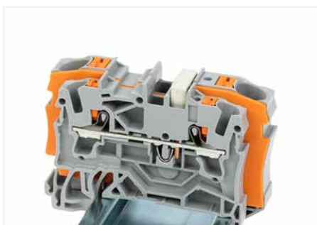
Step-down jumper (Item No. 2006-499) commons 6/4 mm 2 (10/12 AWG) terminal blocks (2206/2204 Series) with 4/2.5/1.5 mm 2 (AWG 12/14/16) terminal blocks (2204/2202/2201 Series).
