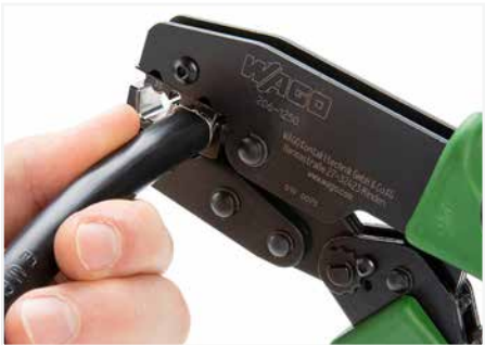
Squeeze handles until ratchet mechanism is released.
