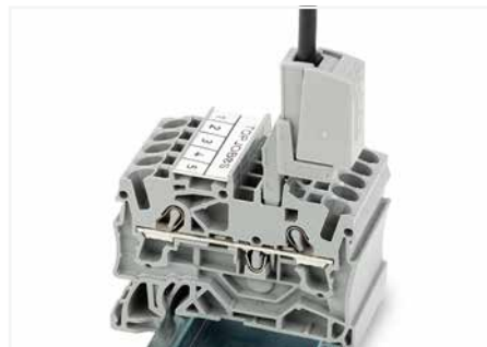
Testing tap (Item no. 2009-182) for tool-free connection of test cables up to 2.5 mm² (12 AWG) – compatible with 2000 to 2016 Series
