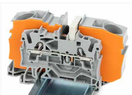
Step-down jumper (Item No. 2016-499) commons 16/10 mm 2 (16/8 AWG) terminal blocks (2016/2010 Series) with 10/6/4/2.5 mm 2 (8/10/12/14 AWG) terminal blocks (2010/2006/2004/2002 Series).
