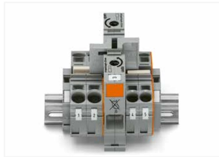
Commoning 35 mm² (2 AWG) POWER CAGE CLAMP Terminal Blocks with 10/16 mm² (8/6 AWG) 2010 and 2016 Series Terminal Blocks TOPJOB® S using step-down jumpers (not valid for Item no. 2016-76xx and 2016-77xx).
