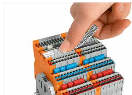
Labeling terminal blocks via marking strips (Item No. 2009-110) or 3.5 mm wide WMB markers (Item No. 793-35xx) – from the top or the side.
