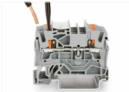
Insert fine-stranded conductors via operating tool.
