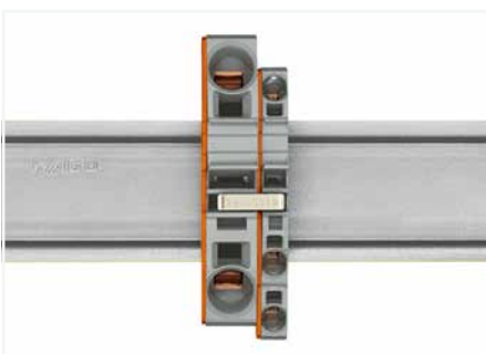
Using step-down jumpers, an end plate must be inserted between the terminal blocks to be commoned.
