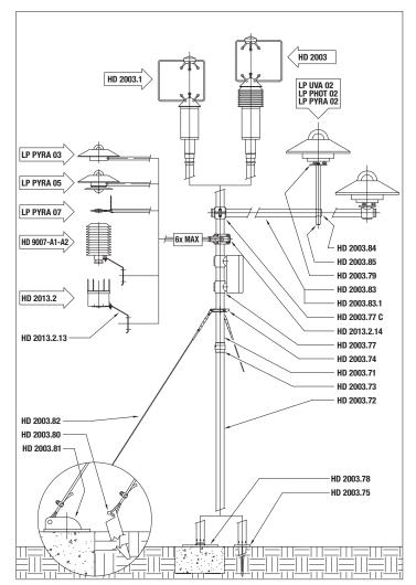
**HD2003.78:** Flange plate for Ø 40mm mast to fasten on the floor
