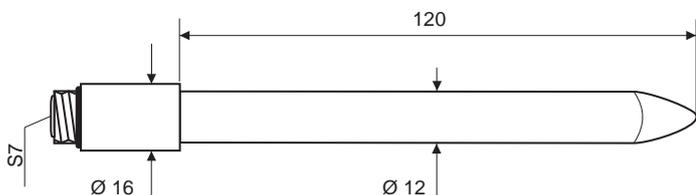
**KP100:** Flat membrane gel combined pH electrode with S7 screw connector, glass body, for skin, leather, paper.
