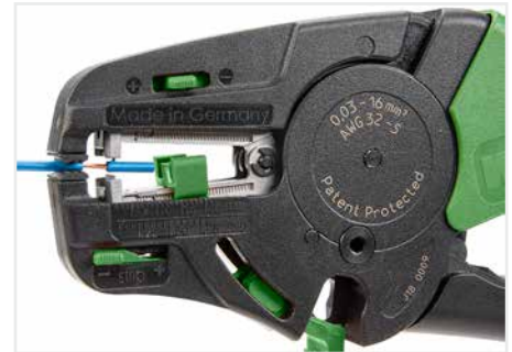
Partially stripping a conductor.
