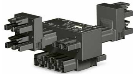
Additional h-distribution connectors double L1 and L3. This results in the following connection option: L1/L1/L2/L2/L3/L3 with jumper in position L2 Notice: h-distribution connectors can only be plugged on L1 and L3.
