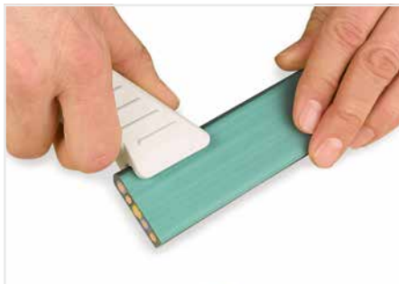
Cut both flat cable insulation sides via stripping knife.
