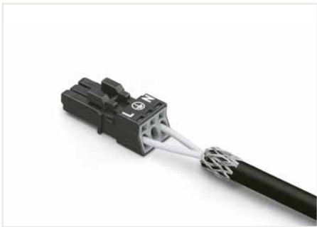
Apply the shield to the rubber cable. Strip length, outer insulation = 40 mm Shield length = 8 mm
