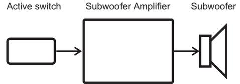
Connect the subwoofer's loudspeaker lead to the loudspeaker connection terminal on the subwoofer amplifier:
