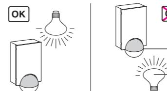
**Minimum distance** Ⓓ between luminaire and movement detector: 5 m. If this distance cannot be achieved, you can use the segments provided to "mask" the light source from the area of detection.
