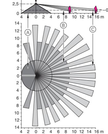
**Inner security zone** Ⓐ: Angle of detection 360° over a radius of approx. 4 m.
