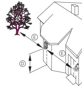
**Mounting height** Ⓑ: 2-3 m. For optimum monitoring, we recommend a height of 2.5 m on a solid and even base.
