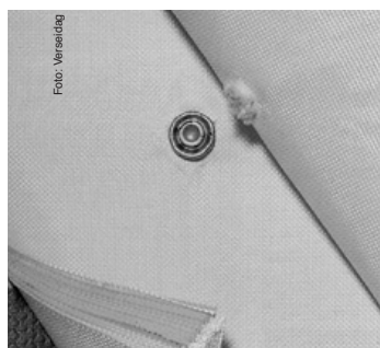
Ballistischer Weichschutz (Kevlar® 29) Soft ballistic protection (Kevlar® 29)
