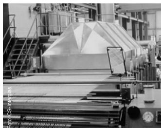
Schlichtemaschine zur Kettherstellung Sizing machine for manufacturing warps
