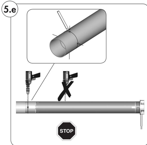
4. Mark the four fastening holes and subsequently drill them through the precision tube in the catch (8).
