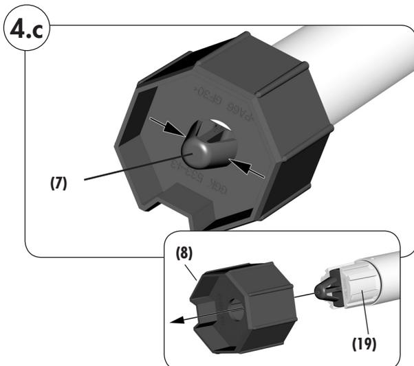
1. Press the side parts of the retaining clip (7) together and pull the catch (8) off of the drive adapter (19).
