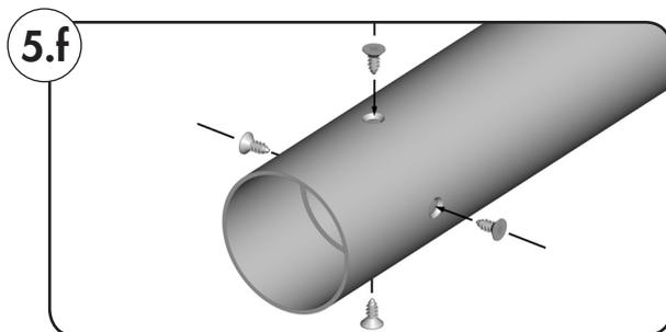
5. Screw or rivet the precision tube to the catch (8).
