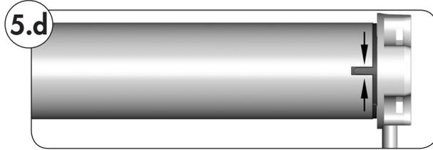
3. Slide the tubular motor into the precision tube.
