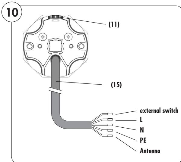
1. Feed the motor cable (15) into the designated junction box or terminal box after hooking the motor in place.
