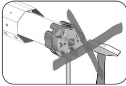
Never knock the motor (9) with force into the rotating union (5). Doing so will cause serious damage.
