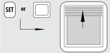
The roller shutters will first travel to the upper stop until the tubular motor switches off automatically.
