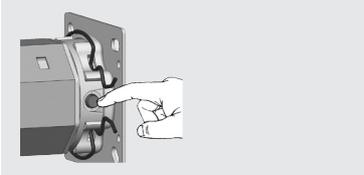
Press and hold the set button (11) until the upper end point is reached.
