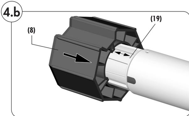
1. Slide the adapter (8) onto the drive adapter (19) so that it cannot free-wheel and so that it engages behind the retaining clip (7).
