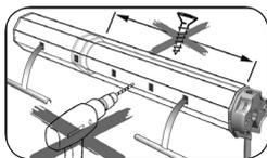
Never drill in the area of the drive or insert screws in order to secure the roller shutters.
