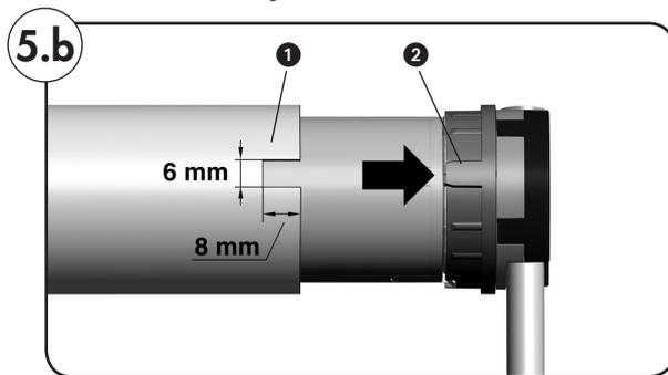
2. Saw a groove in the end of the precision tube 1 in order that the cam 2 of the adapter (10) can be pressed fully into the tube.
