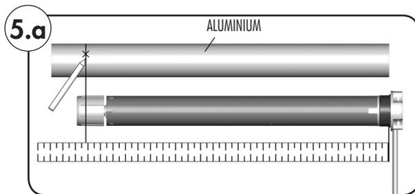
1. Measure the distance between the adapter (10) and the rear third of the catch (8) and mark this distance on the precision tube.
