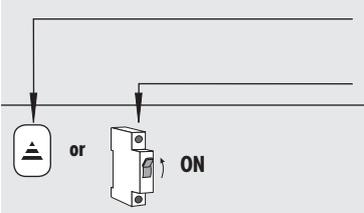
Symbols and actions when connecting a cord circuit setting unit (22) or when connecting an external switch.
