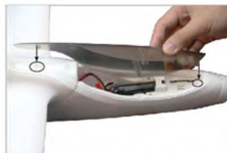
9. Lay the canopy, aim into the buckles
