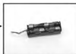
According to the correct polarities, install 8 x AA battery
