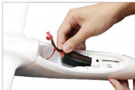
7. Insert the battery into the compartment
