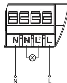
→ If the terminal needs to be disconnected, press the lock with a suitable screwdriver. Afterwards, the cable can be pulled out again.
