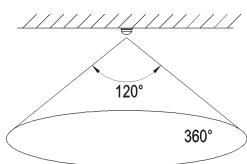
The range for detecting a temperature change in the detection range depends on several factors:
