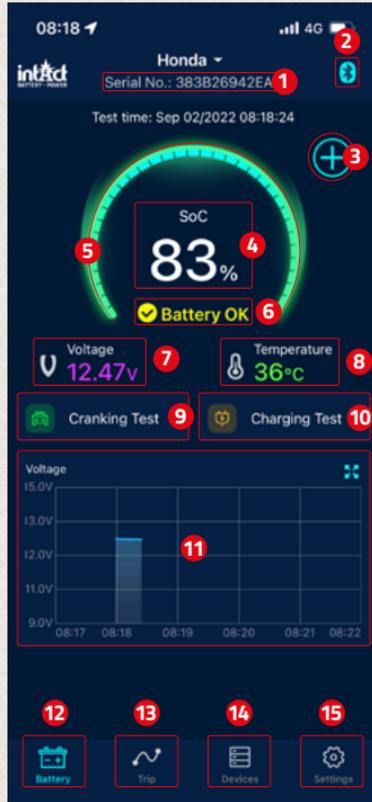
11. Battery voltage history graph: Click on the graph to enlarge it. The graph shows you either the state of charge in %, the temperature or the battery voltage in volts. Here you can choose between the display of one day, 3 or 5 days. You can also switch between the days at the top center.
