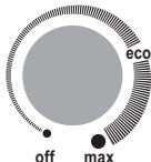
► To **increase** the cooling capacity, turn the cooling capacity control clockwise.
