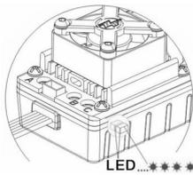
→ The sound signal is caused by briefly activation of the brushless motor. However, depending on the motor it can be very muted or you may not hear it. In this case, pay attention to the LEDs on the speed controller.
