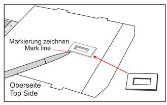
Using a ruler and sharp knife, carefully cut through and remove the covering film as shown.
