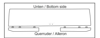
Test fit the ailerons to the wing with the hinges. If the hinges don't remain centered, stick a pin through the middle of the hinge to hold it in position.
