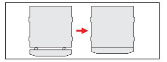
Put the horizontal into the fuselage. Check the fit of the horizontal stabilizer in its slot. Make sure the horizontal stabilizer is square and centered to the fuselage by taking measurements, but don't glue anything yet.
