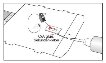
Place the servo into the servo tray. Center the servo within the tray and drill 1.5mm pilot holes through the block of wood for each of the four mounting screws provided with the servo.
