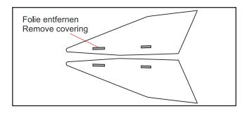
Using a modeling knife, remove the covering on the slot of the vertical stabilizer. Mix up a generous amount of 30 minute epoxy. Apply a thin layer to the slot in the vertical stabilizer. Slide the vertical stabilize into the mounting platform of the horizontal stabilize. Using a triangle, check to ensure that the vertical stabilizer is aligned 90 degree to the horizontal.
