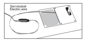
Place the servo into the servo tray. Center the servo within the tray and drill 1.5mm pilot holes through the block of wood for each of the four mounting screws provided with the servo.
