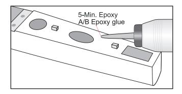
After the epoxy has fully cured, remove the masking tape or T-pins used to hold the stabilizer in place and carefully inspect the glue joints. Use more epoxy to fill in any gaps that may exits that were not filled previously and clean up the excess using a paper towel and rubbing alcohol.
