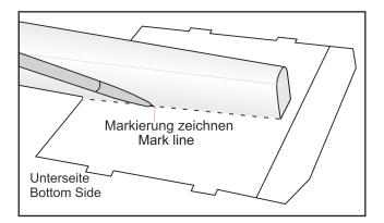
Remove the stabilizer. Using the lines you just drew as a guide, carefully remove the covering from between them on the bottom of the tail plane using a modeling knife.
