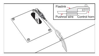
Repeat the procedure to install the second aileron.
