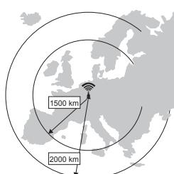
If the DCF signal was received properly, the weekly timer synchronises the clock daily by several signal searches in the night (at 2 a.m., 4 a.m. and 6 a.m.), since there is the least interference from other electric/electronic devices.
