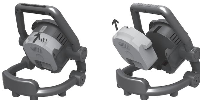
The battery can be easily and quickly replaced. Press the lock (F) forward and then slide the battery up and out, see drawing. It is therefore possible to charge one battery and continue working with a separately available replacement battery.
