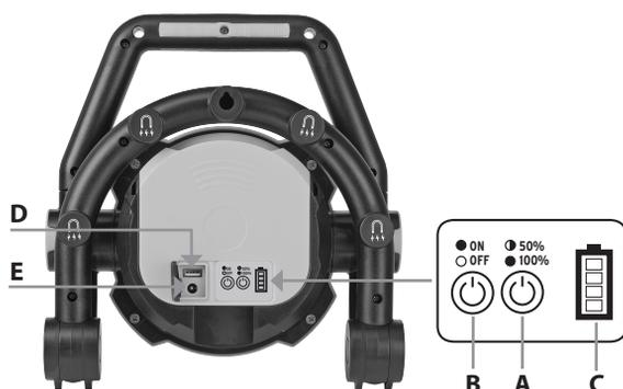
Press the (B) button to turn on the lamp. By pressing the (A) button, the brightness can be set to 100% or 50%.
