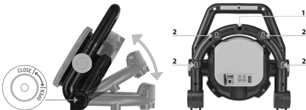
For set-up, the battery-operated lamp can be unfolded to several settings, but, at most, to the "OPEN" marking. Do not force the lamp further open since this would damage the mechanism! The lamp can be hung up on a hook on the frame using the mounting opening (1) or on a metal surface using the magnets (2). Please make sure the surface is stable in order to avoid damage to the product or injuries to persons!
