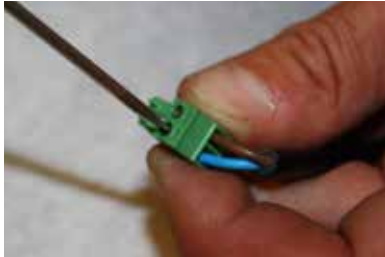
Mount cables and tighten screws
