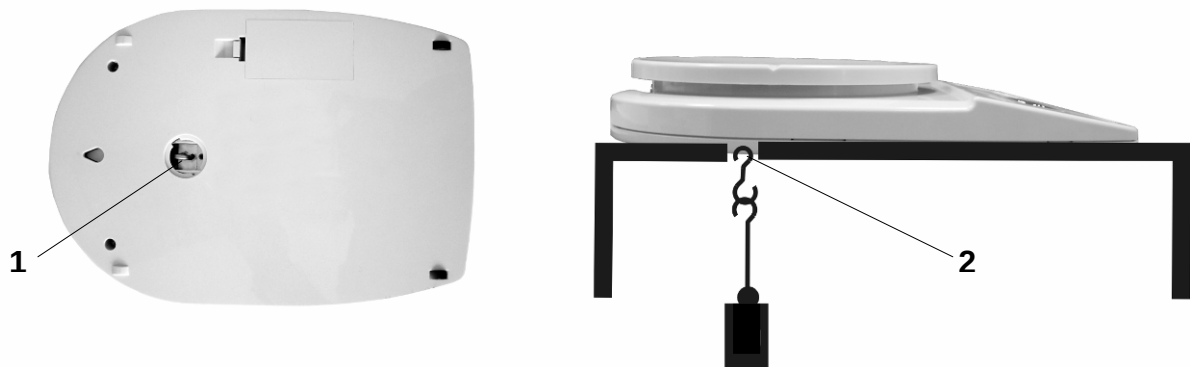
Fig. 1: Setting up the balance for underfloor weighings
