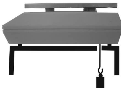
Fig. 1: Setup of balance for underfloor weighing
