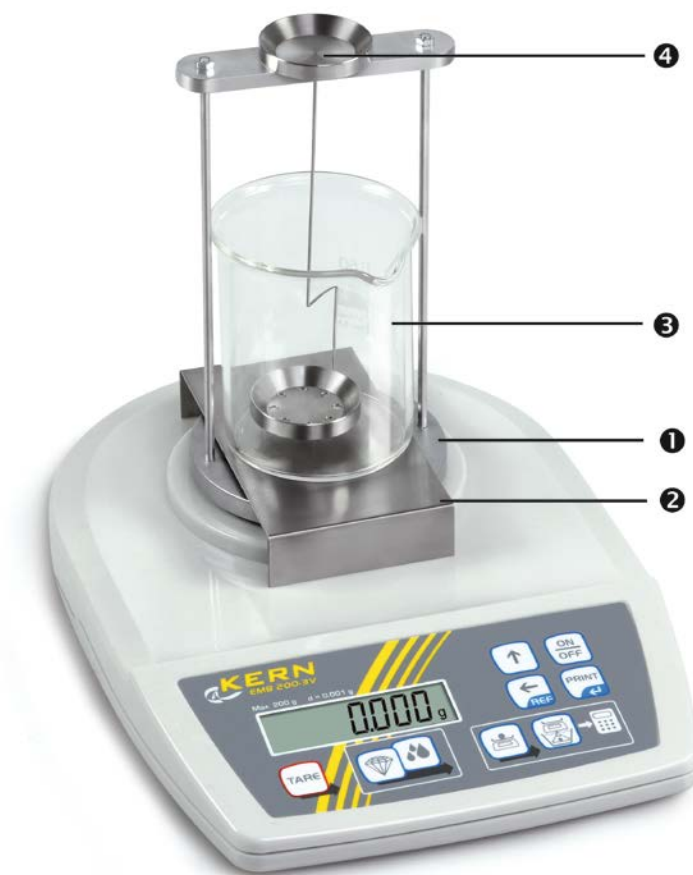
Fig.1: KERN EMB 200-3V with installed density sets KERN YDB-01 (numbering, see chap. 1)
