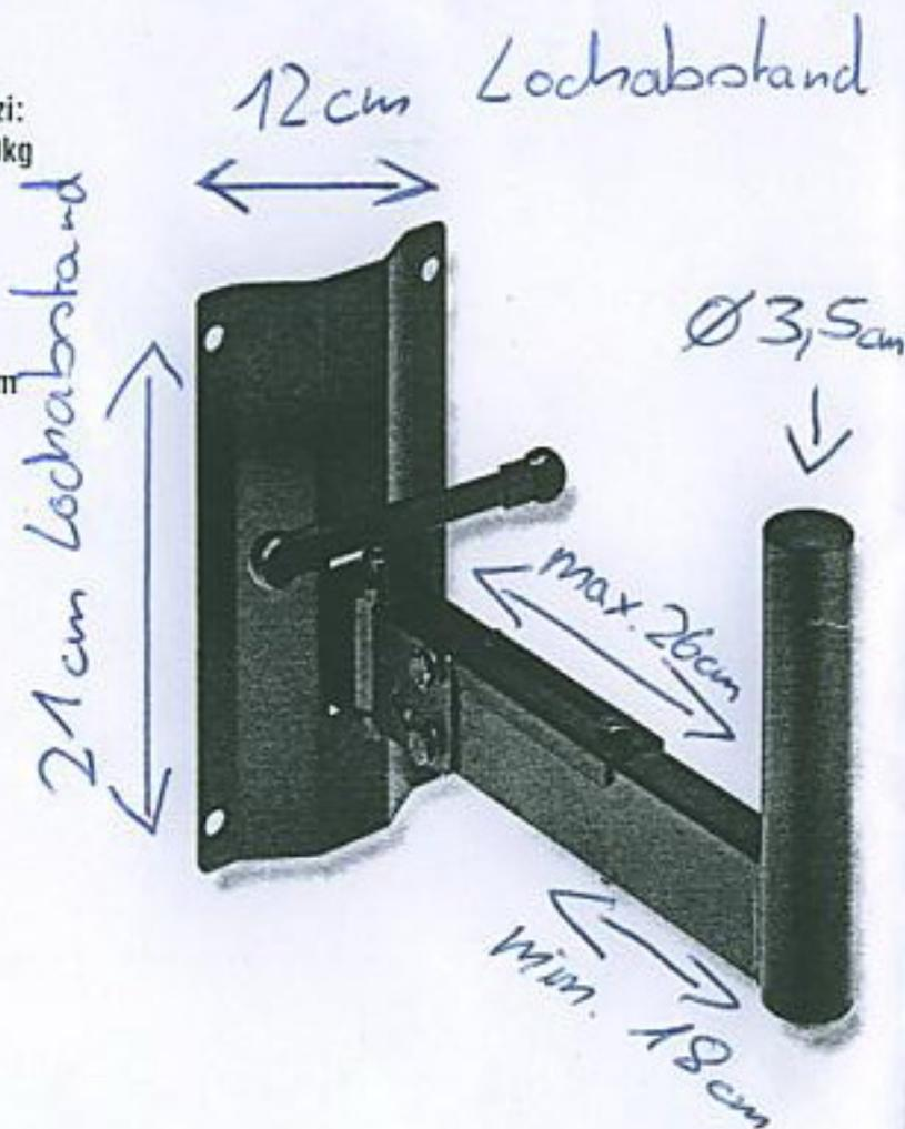
Adjustable wall mounting bracket with arm L=260mm and male attachment H=120mm,  $\varnothing$  35mm to hold speaker. The arm with an adjustable support to clamp the speaker swivels in the horizontal plane and may be tilted. Position of support from centre of male attachment: min. 180mm, max. 260mm. Wall plate 250x140mm with 4 holes  $\varnothing$  10mm to fix bracket.
