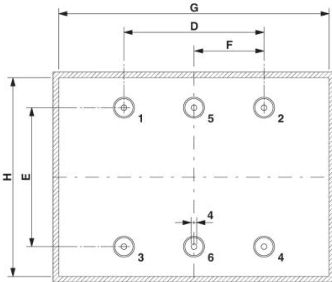
Mass D: 100,0 mm; E: 80,0 mm; G: 160,0 mm; H: 112,0 mm
