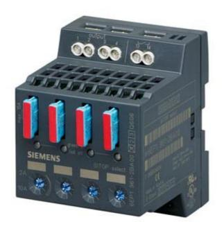
SITOP SELECT DIAGNOSEMODUL 4-KANALIG EINGANG: DC 24 V AUSGANG: DC 24 V/10 A JE KANAL AUSGANGSSTROM EINSTELLBAR 2-10
