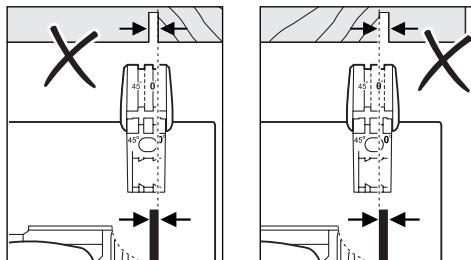
For precise cuts, position the circular saw against the workpiece as shown in the figure. It is best to carry out a trial cut.
