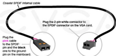
Plug the **pink** cable to the SPDIF-pin and the **black** one to the ground-pin on the mainboard.
