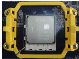
2. Align Pin-1 of the CPU with the CPU socket, and gently put the CPU onto the socket.
