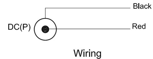
Voltage/Current Max.:12VDC 3A
