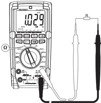
→ If you carry out a resistance measurement, make sure that the measuring points you touch with the measuring prods are free from dirt, oil, solderable lacquer or similar. Such circumstances can falsify the measured result.
