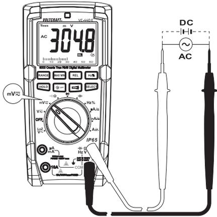
→ The voltage range “mV” has an input resistance of  $\geq 10\text{ M}\Omega$ . With the measuring inputs open, the high sensitivity may cause an undefined measured value to be displayed; however, this does not influence the measuring result.
