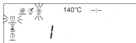
The currently set heating profile and switch-off criterion flashes.
