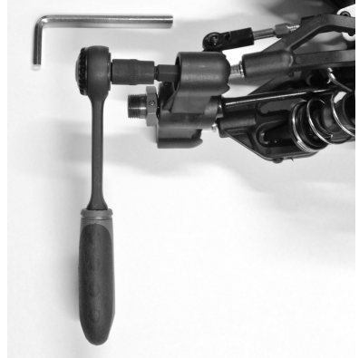
Tightening/loosening the set screw (C)
