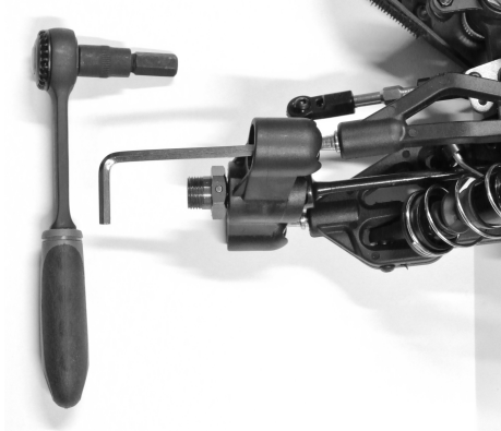
Adjusting the spherical-head screws (A and B)
