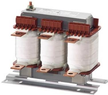
NETZDROSSEL F. FU; PHASEN:3; UN1(V):480; ITHMAX 1(A) / F1(HZ):63 /60; I LN (A):56,7; UK(%):2; LN(MH):0,224; TA/ISOKL:40 /B; IP00; ANSCHLUSS:FLACHANSCHLUSS; EN 61558-2-20 >UL/CSA-RECOGNIZED< >DROSSEL<
