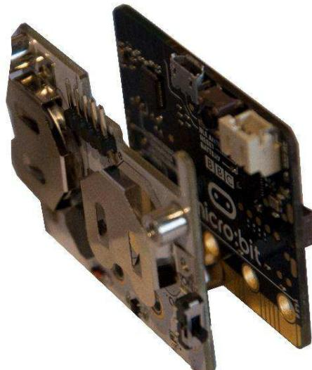
Screw the Power:bit and micro:bit boards together. Do the same for pins 1, 2 and 3V.
