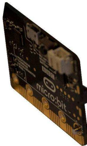
Line up the Power:bit board with the screws. The back of the Power:bit must face the back of the micro:bit.
