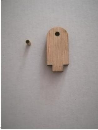
A photograph showing two small wooden parts: a small cylindrical piece and a larger, U-shaped wooden piece with a hole in the center, both on a light-colored surface.                                                                                                                                      | <p>Radaufhängung und Messinghüse (kurz)</p>                                                                                 |
