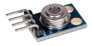
This infrared sensor module uses the MLX90614 sensor and enables non-contact temperature measurements. The control is particularly simple via the I2C interface and is thus possible with a wide variety of microcontrollers and single-board computers.
