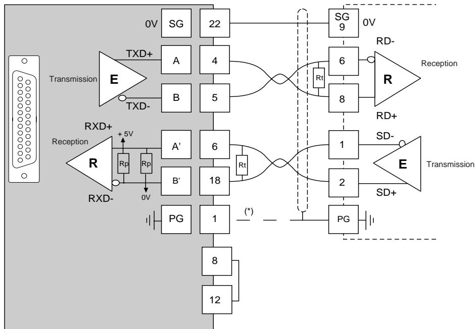
\* The connection of the shielding to both cable ends depends on the electrical operating conditions.
