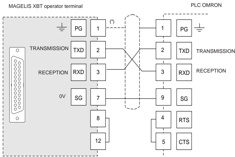
\* The connection of the shielding to both cable ends depends on the electrical operating conditions.
