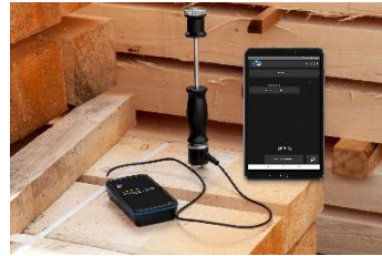
Figure 3 PCE-WMT 200 with measuring electrode
