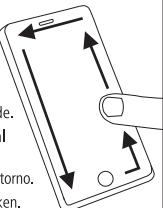
**EN** This glass uses contact small spots and does not adhere over the full surface but only on the edges. After positioning and removal of the protective layer, just press firmly on the edges circumferential for fixation.
