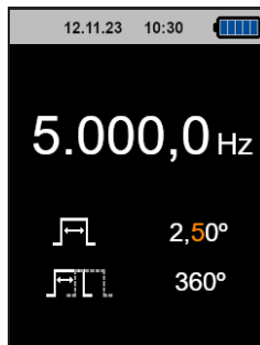
Figure 32. Quick mode - duty cycle modification
