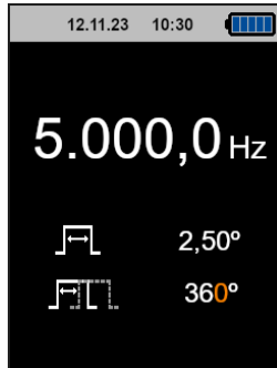
Figure 33. Quick mode - phase shift modification
