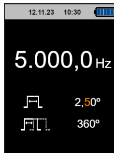
Figure 32. Quick mode - duty cycle modification
