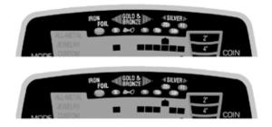
All Notch Discrimination modifications made while in the CUSTOM mode will be retained when the detector is turned OFF. However, all changes made to the Notch Discrimination scale while in the ALL-METAL, JEWELRY, RELICS
