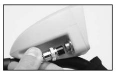
The location of the arm cuff may be adjusted by removing the screw on the bottom and moving it to the other hole.
