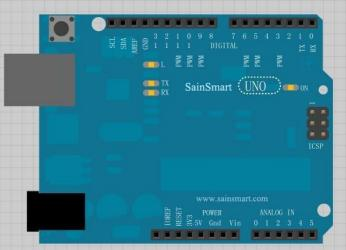
Accordance with the good circuit after the link above figure, you can start writing programs, and we let the small LED lights flashing. Lighting on for one second and off for one second. This program is very simple. This is Arduino own routines Blink.
