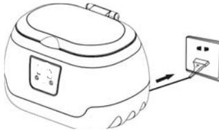
2. Close the lid. Connect the unit with power. **The blue light on the lid will be on for viewing**
