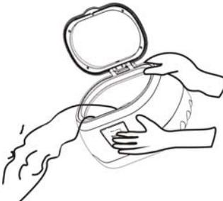
4. When cleaning is over, cut off the power. Open the cover, take the cleaned article out and drain the water
