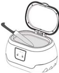
For large articles, partly cleaning as shown.
