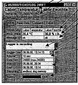
Identification: (only if supported by logger) can be altered under 'extras' and will be stored in the logger
