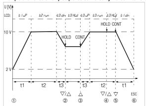
**Ramp parameters:** output quantity: U (range of 0 ... 15 V),  $5 \pm Rr \pm 2$  V, Erd = 10 V, Erd = 5 s, Erd = 8 s, Erd = 5 s, erd = 10 V, Erd = 10
