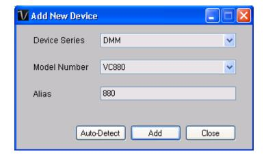
Enter a unique alias for this device, click "Add" will add the device into Voltsoft. User may also launch this module by selecting Device Management->Add New Device in menu.
