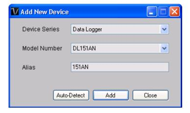
Enter a unique alias for this device, click "Add" will add the device into Voltsoft. User may also launch this module by select Device Management->Add New Device in menu.
