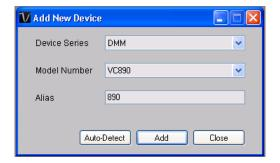
Enter a unique alias for this device, click "Add" will add the device into Voltsoft. User may also launch this module by select Device Management->Add New Device in menu.
